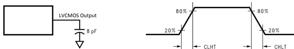
Figure 2. LVC MOS Output Load and Transition Times
