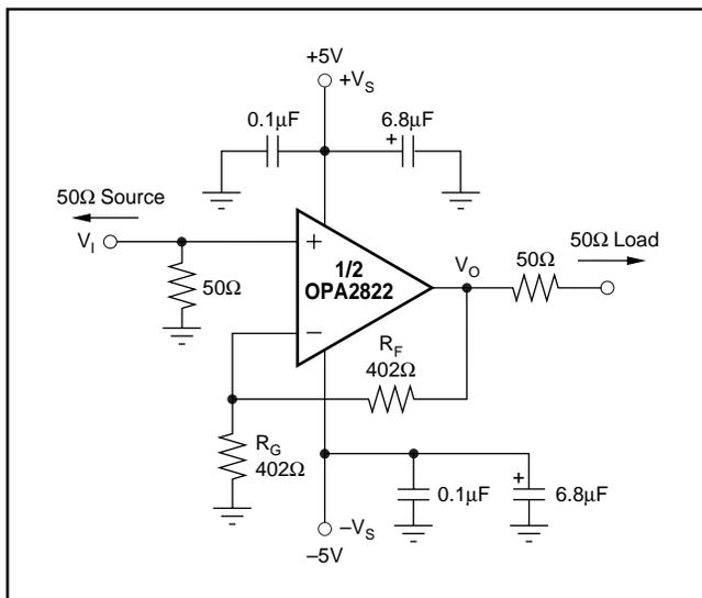
FIGURE 1. Noninverting  $G = +2$  Specification and Test Circuit.
