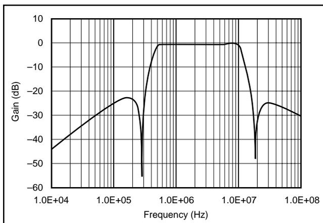
FIGURE 7. Frequency Response for the Filter in Figure 6.
