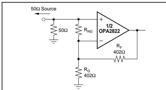
FIGURE 12. Noise Gain Tuning for Noninverting Circuit.
