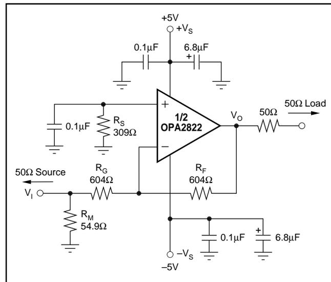
FIGURE 2. Inverting  $G = -1$  Specification and Test Circuit.
