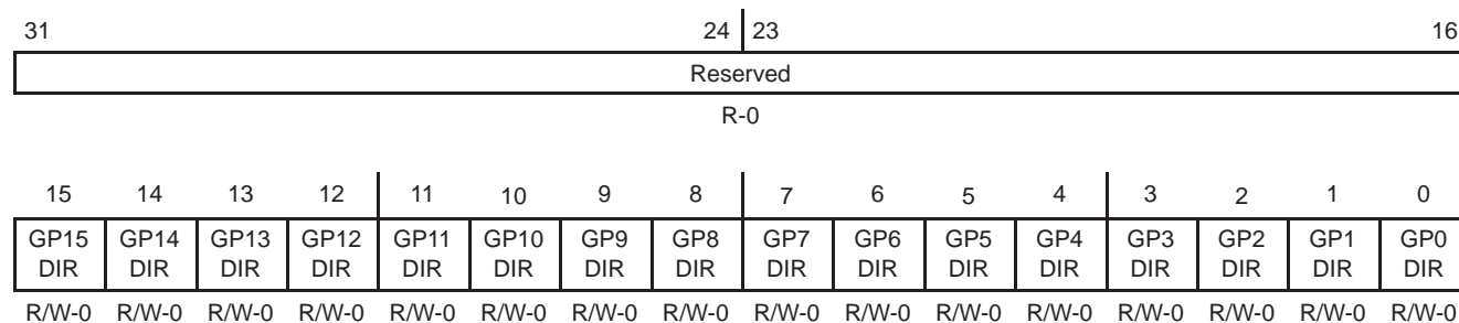
Figure 7. GPIO Direction Register (GPDIR) [Hex Address: 01B0 0004]
