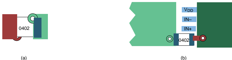
Figure 48. Typical Decoupling Capacitor Layouts
