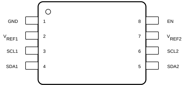
图 5-1. DCU Package, 8-Pin VSSOP, Top View
