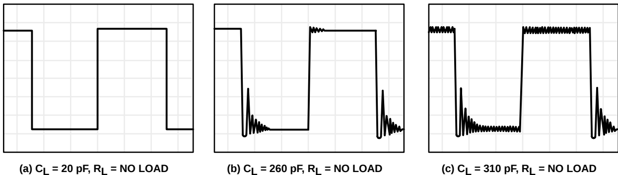
Figure 112. Effect of Capacitive Loads in Low-Bias Mode
