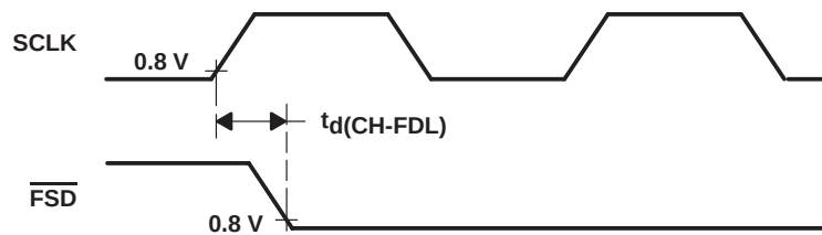
Figure 5–3. Master/Slave SCLK to \overline{FSD} Timing
