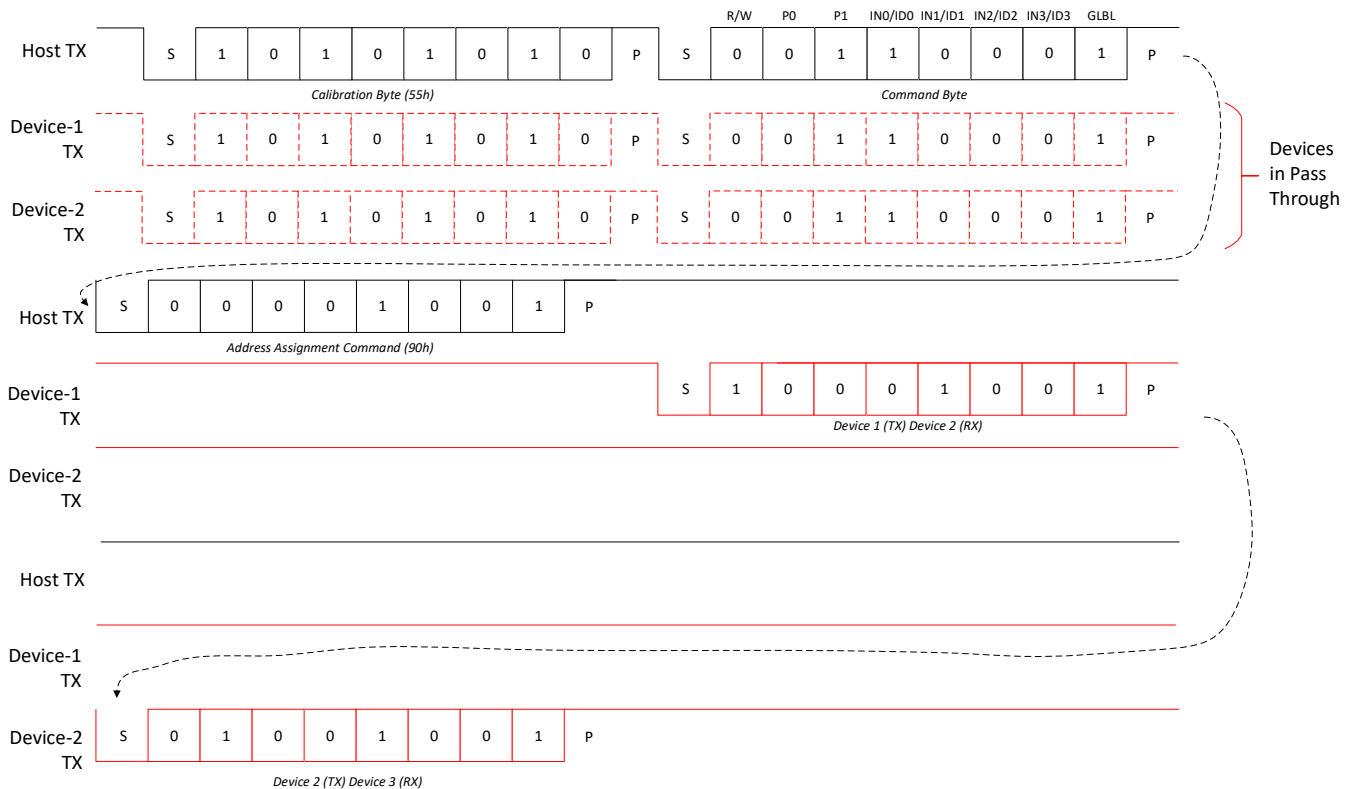
图 7-8. Global Initialization and Address Assignment Command Flow
