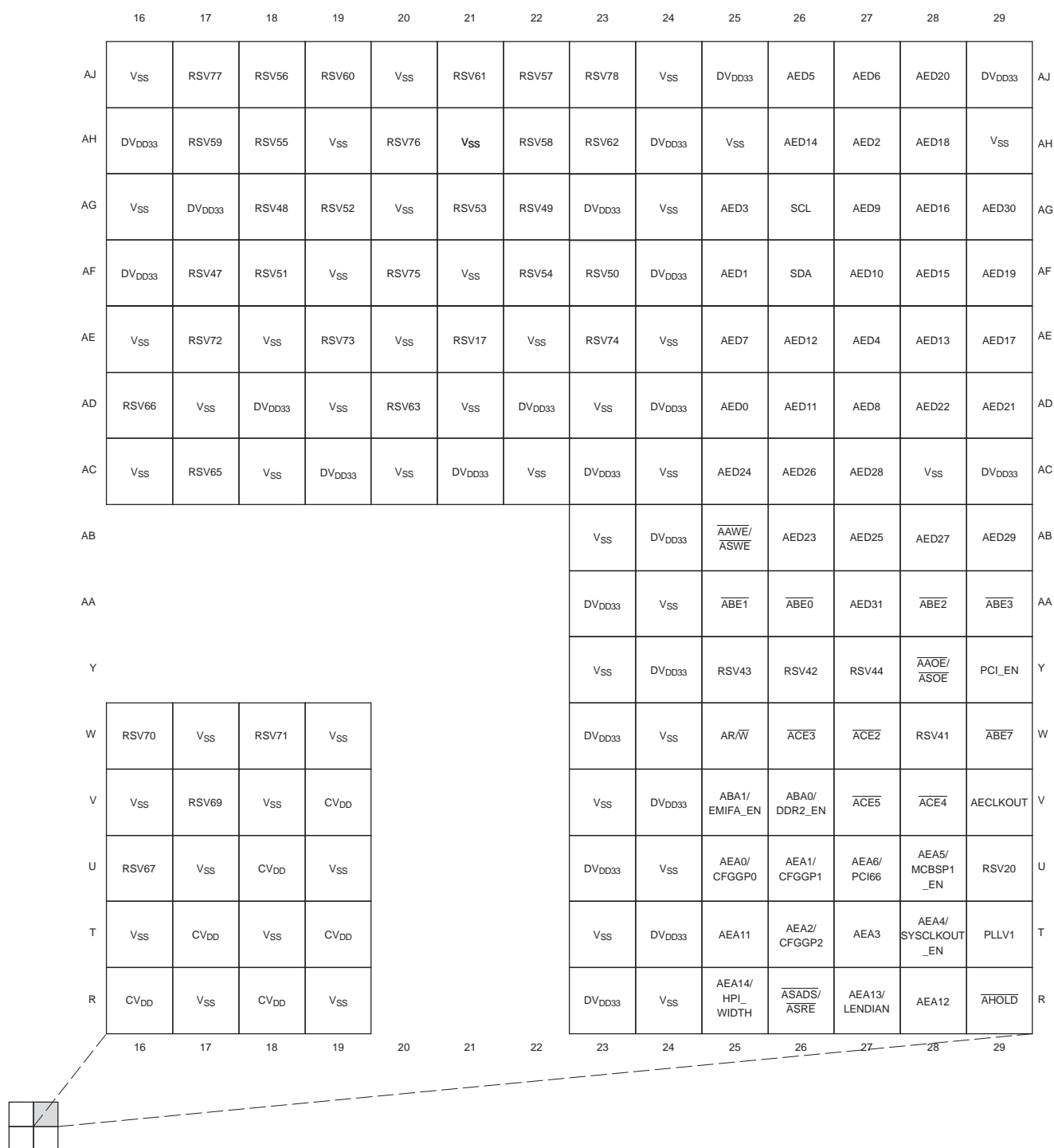
Figure 2-3. C6454 Pin Map (Bottom View) [Quadrant B]
