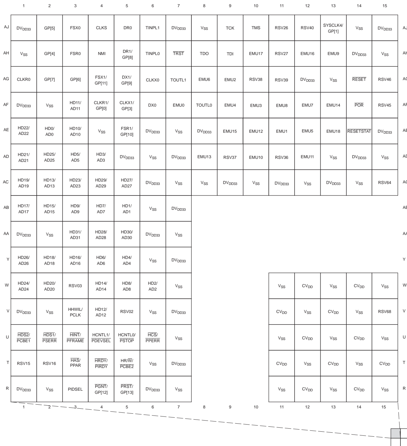
Figure 2-2. C6454 Pin Map (Bottom View) [Quadrant A]
