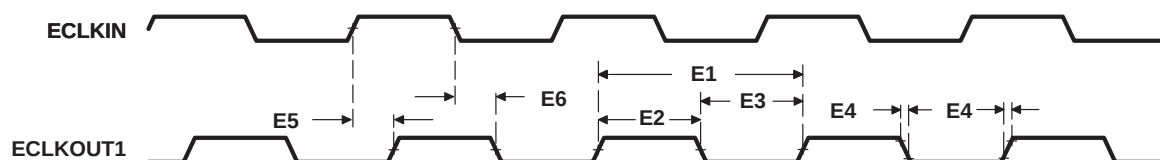
Figure 5–6. ECLKOUT1 Timings for EMIF Module
