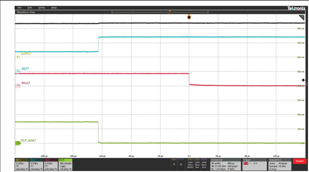
图 6-14. LED Open Protection
