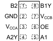
图 6-2. DTT Package, 8-Pin SON Transparent (Top View)
