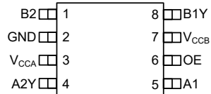
图 6-1. DCU Package, 8-Pin VSSOP (Top View)
