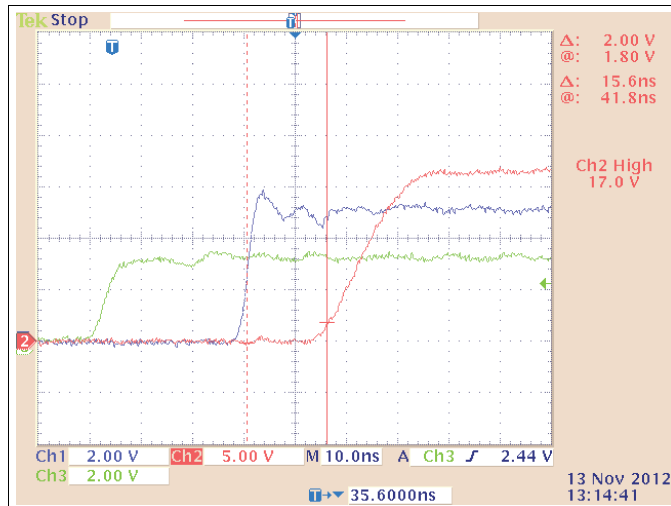
图 42. UCC27531DBV Input vs. Output PWM Propagation Delay (High)
